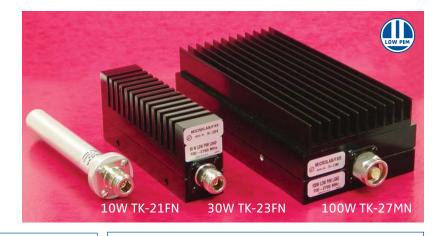
Microlab TK-20 series Low PIM Cable Loads cover from 10 to 200W average power. They are intended for wireless applications, when extremely low PIM, Passive Intermodulation, is required. A typical application is in terminating the unused port of a Hybrid Coupler used to combine different wireless signals. These are also offered as a discrete products in the CT series.
